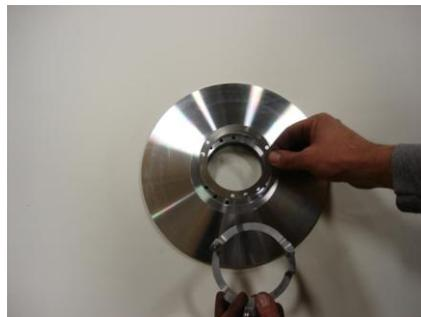
**NOTE: MAKE SURE THAT THIS BUSHING RETAINER SHIM IS INSTALLED. IF THIS SHIM IS LEFT OUT OF THE DRIVEN CLUTCH , THE MOVABLE BUSHING WILL WORK ITSELF OUT AND YOU WILL DAMAGE YOUR CLUTCH!**
