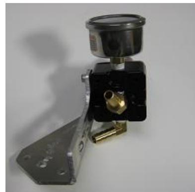
side of the pressure regulator. The center port on the back side is the fuel return back to the top R.H. corner of fuel tank. Then use Teflon tape on the fuel pressure gauge and install it into the top side port of the pressure regulator. Clock the pressure regulator so it positions the hose barb at about the 4 o'clock position, then install the pressure regulator onto the aluminum pressure
