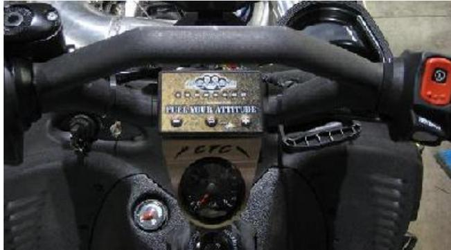
models that have the telescoping handlebars, you will need to take a round file or a die grinder with a carbide burr and widen the mounting holes in the boost bracket and you will need to install longer Stainless steel 8m X 40m bolts and washers to space the boost bracket to the handlebar clamp to hold the boost bracket on. We also have in stock a optional two hole gauge stainless steel bracket if you want to install more gauges as well as custom brackets for EGT gauges.
