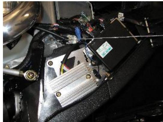
reinstall Phillips head screw into the side tab. On 2009 models, you will need to drill a 1/4 inch hole through this bracket to mount the stock voltage regulator in the stock position on top of this bracket. Next re-mount the air temp sender onto the top side of this new bracket. Re-attach the blue/black wires to the main wiring harness.
