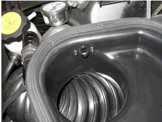
1/2 inch drill bit and drill a hole in the bottom of the 4" X 3" rubber elbow to allow water to drain out. The hole is located in the rubber hose at the lowest point in the hose, close to the inlet of the turbo charger. **If this step is not performed, water could puddle and freeze, turning to ice and damage the compressor wheel of the turbo.**
