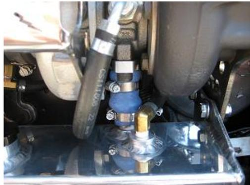
from the supplied parts, find two washers that have a 14m rubber seal in the inside diameter and twist the metal/rubber washers on to two (2) of the fitting that have male threads on them; the end that has 14m threads is where the metal/rubber washer is placed. Then this fitting is screwed into the center section of the turbo.
