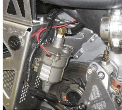
Before permanently mounting the oil pump to the foot rest, you will need to connect the oil line hoses to the oil pump. The oil line that is 5/16 X 19 inches long that feeds to the top of the turbo, must be connected to the top of the oil pump outlet (this is the same hose as in instruction #13 above). The bottom brass oil pump barb
